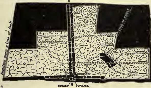
FIG. 7.—Long-wall method of working Coal in Derbyshire.
